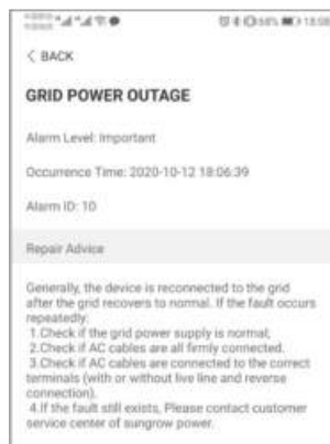
Figure 7-10 Detailed Fault Alarm Information
