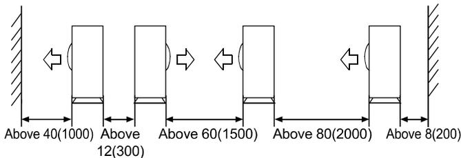
The top and two side surfaces must be exposed to open space, and barriers on at least one side of the front and back shall be lower than the outdoor unit.
