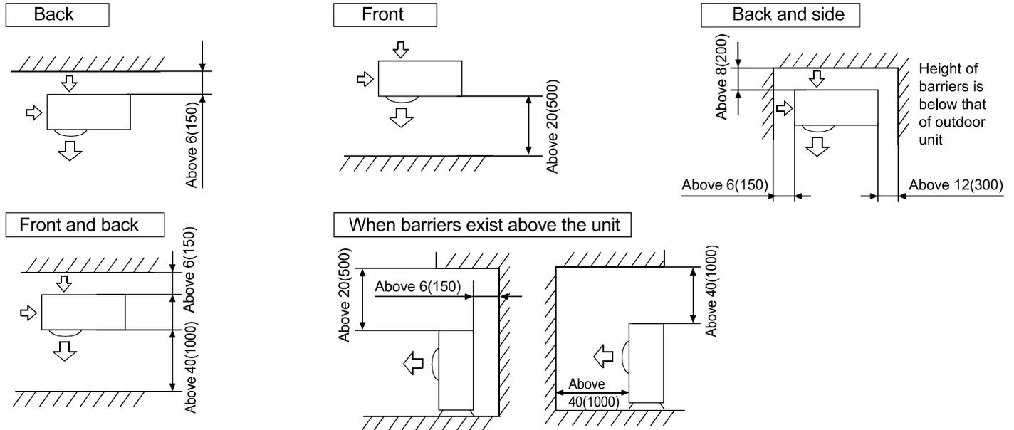
The top and two side surfaces must be exposed to open space, and barriers on at least one side of the front and back shall be lower than the outdoor unit.
