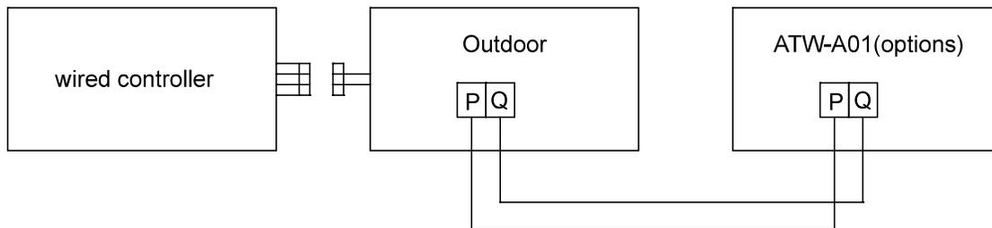
The outdoor and ATW-A01 units are in parallel through 2 non-polar wires.
